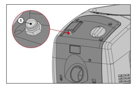
The fuse **(1)** protects the socket against overload due to overcurrent. When it responds, a white pin becomes visible under the transparent cap. Pushing the pin will turn the power back on.
