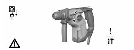
Set the function selector switch to the "Hammer drilling" position T.
