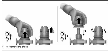
5.3 Fitting / removing the accessory tool
